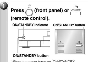
When the power turns on, ON/STANDBY indicator on the front panel changes color from red (standby mode) to green (operation).
