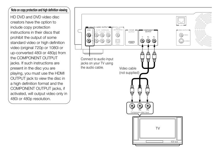
Switching output signals (Switching to component video output and setting the resolution)
